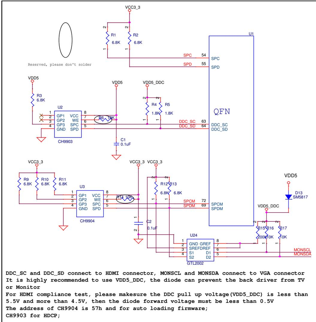
Figure 7: Serial Port Interface: DDC\_SC, DDC\_SD, SPCM, SPDM and SPC, SPD pins of CH7033B and CH7051B
