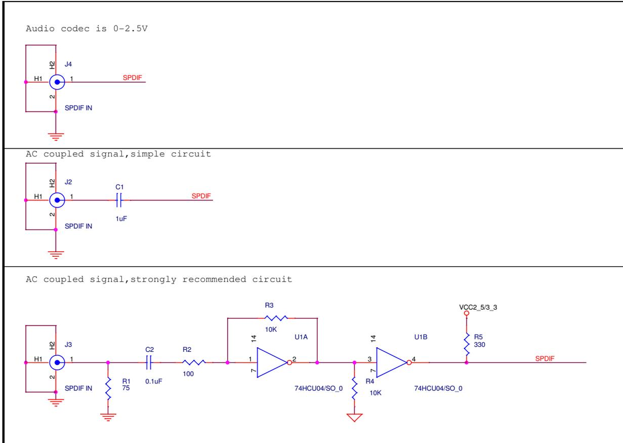
Figure 9: SPDIF pin of CH7033B and CH7051B
