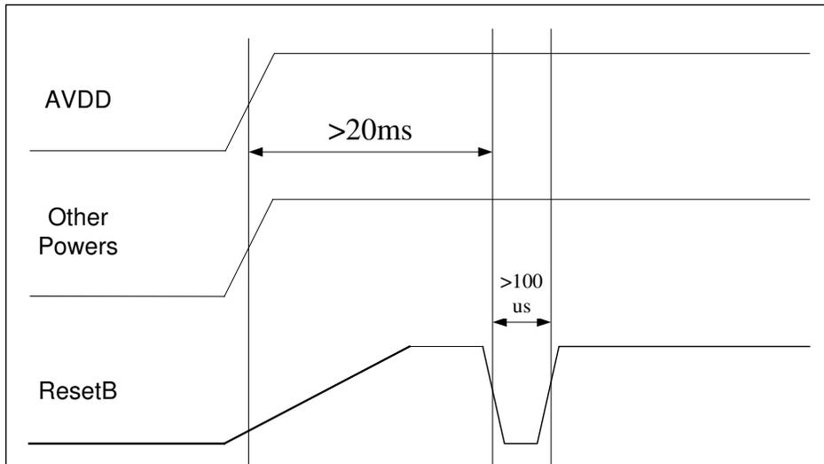
Figure 3: Power-on Reset Function's Sequence external global reset
