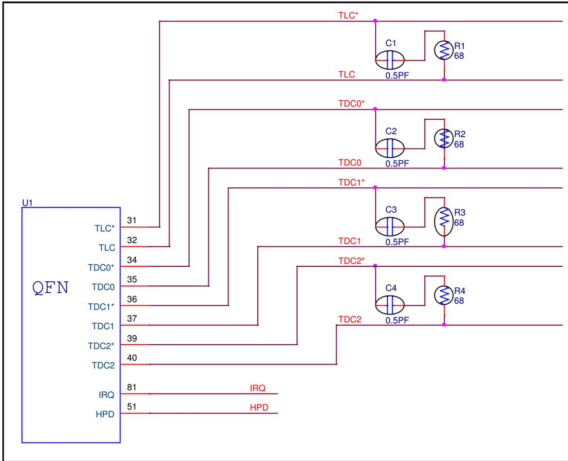
**Figure 11(A): The connection of the DVI/HDMI outputs**
