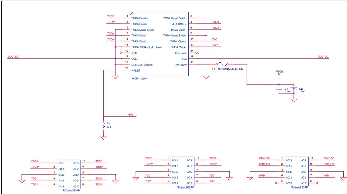
**Figure 11(B): The connection of the HDMI outputs—CH7033B and CH7051B HDMI connectors**
