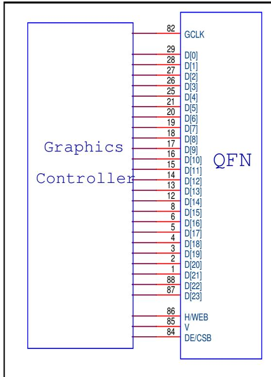
Figure 8: CH7033B and CH7051B Data Input Pins
