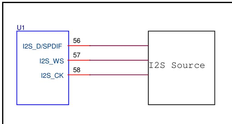
Figure 10: CH7033B and CH7051B I2S Input Pins
