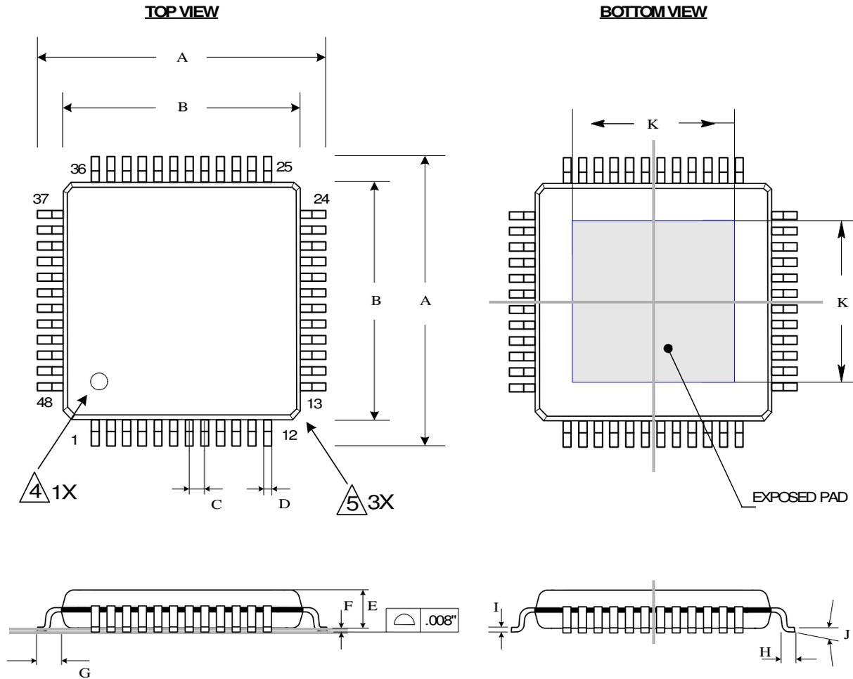
Figure 5: 48 Pin LQFP (Exposed Pad) Package
